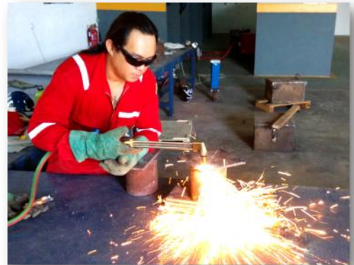
Oxy-Acetylene Cutting In Progress
